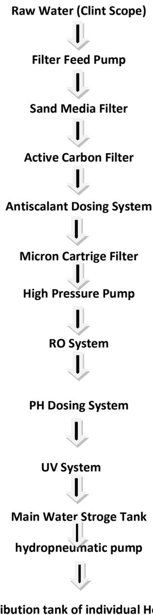
The Reverse Osmosis system works on the Principle of the natural phenomenon of OSMOSIS PROCESS. Since OSMOSIS PROCESS is reversed by external pressure the process is termed as REVERSE OSMOSIS. Reverse Osmosis is a water purification process in which water is forced by pressure through a semi-permeable membrane.
