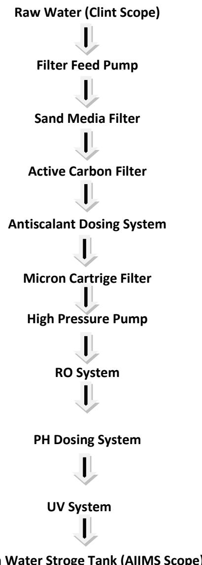
The Reverse Osmosis system works on the Principle of the natural phenomenon of OSMOSIS PROCESS. Since OSMOSIS PROCESS is reversed by external pressure the process is termed as REVERSE OSMOSIS. Reverse Osmosis is a water purification process in which water is forced by pressure through a semi-permeable membrane.
